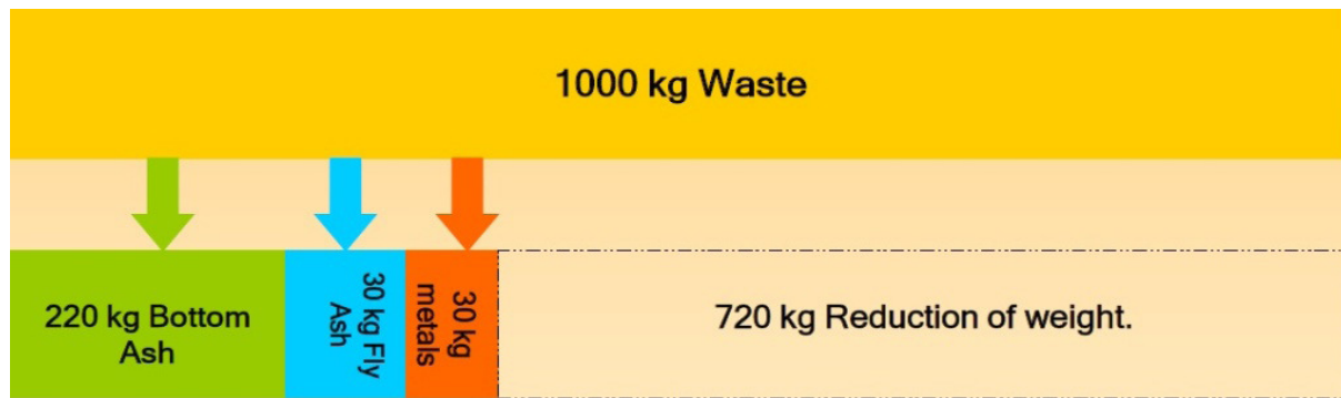
Figure 10. Mass balance of an incineration plant.
