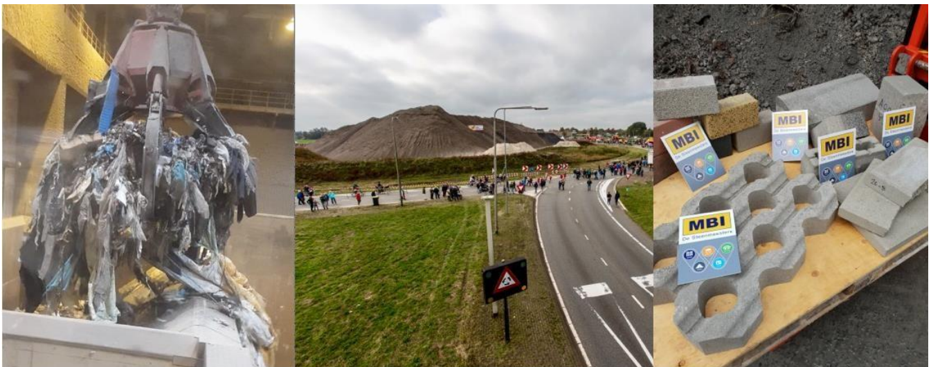
Figure 1. Waste handling crane in Reststoffen Energie Centrale plant, and examples of "useful" applications of bottom ash, October 2019 (photos: K. Bouman), mountain of bottom ash in Joure 2019 (photo Jaring Rispens)
