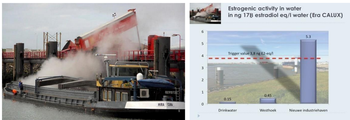
Figure 3. Transshipping bottom ash in cargo ships Harlingen (2011) and the results Era-CALUX of water spoiled with bottom ash (2014).
